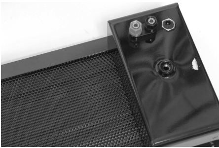
A. The electronics housing is at one side of the panel
